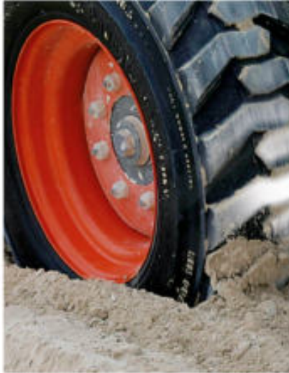
CUVED LUGS IMPROVING TIRE CLEANOUT
