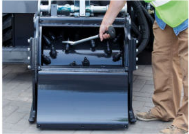
6678074 Bit removal hammer punch
