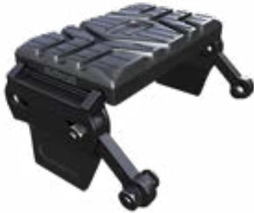
These tracks are designed for serious traction and rough conditions. The diamond pattern creates more traction than normal smooth bar tracks, maximizing your machine's power. The track design allows excellent clean-out for snowy and icy conditions or mud and clay.
