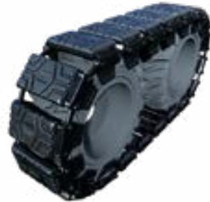
Rubber over-the-tire tracks are extremely versatile and allow you to maximize your traction without damaging surfaces like pavement, asphalt or grass. They also provide excellent flotation and traction in muddy or slippery conditions.
