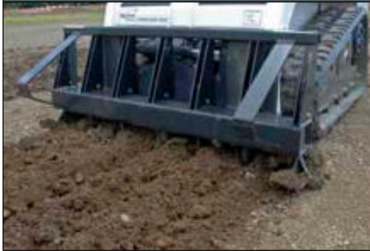
Scarifier: Includes 2 Depth Guides and 5 teeth.
