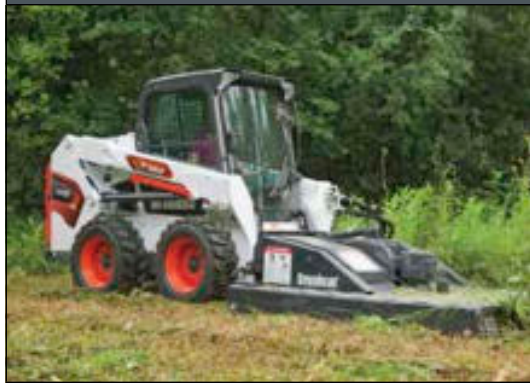
Brushcat™ Rotary Cutter: Comes standard with a 7 cm Offset Blade and Front Wheels. Cutting height of 7.6 cm.
