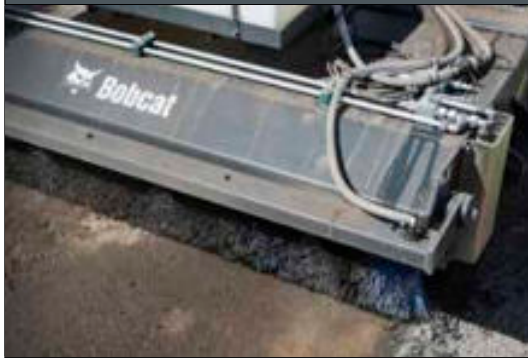
Sweeper: Machine must have front hydraulic auxiliary.
