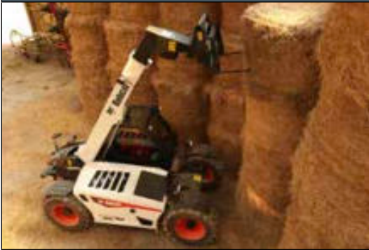
Bale Fork: To be mounted on rigid fork frame.
