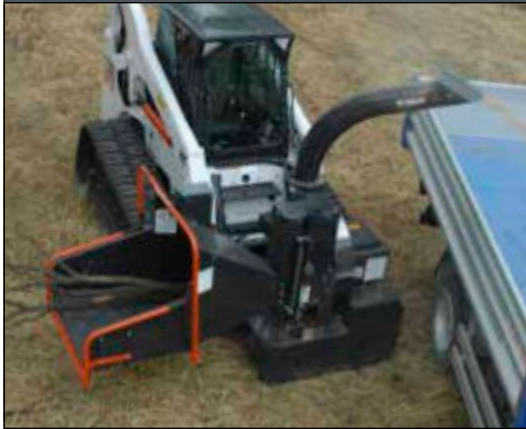
Wood Chipper: Loader must be equipped with a 7-Pin Control Kit.
