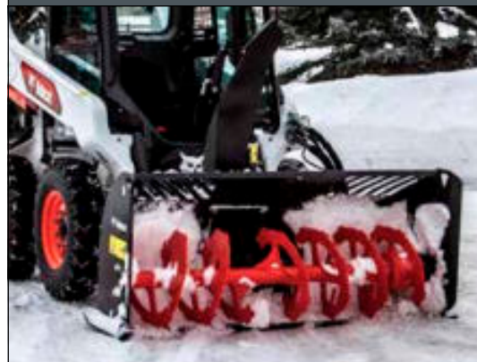
Snow Blower: Includes a hydraulic motor package. Loader must be equipped with a 7-pin Attachment Control Kit.
