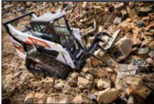
Industrial Grapple: Includes Bolt-On Cutting Edge. It is recommended to use a port relief valve.
