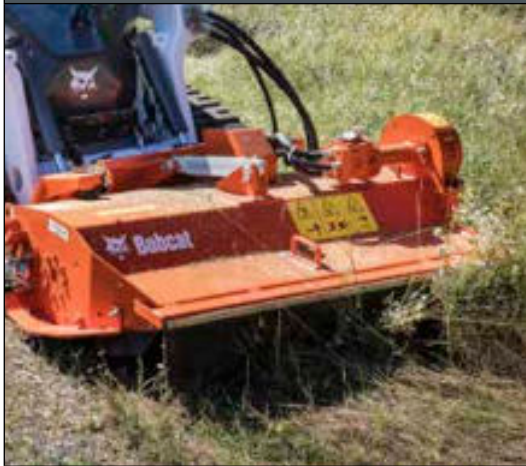
Flail Cutter: Machine must have front hydraulic auxiliary.
