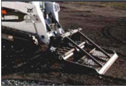
Landplane: Includes expanded metal grate, scarifier assembly, teeth and respective hardware.
