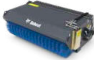
Sweeper: Machine must have front hydraulic auxiliary.
